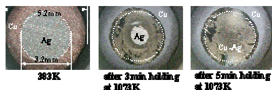
Fig.2 High-temperature microscope pattern of melting during heating of an Ag-Cu binary bonding system.
