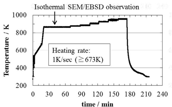
Fig.1. Heat pattern of *in-situ* SEM/EBSD.
