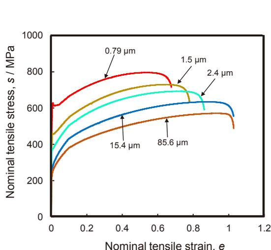
Fig. 2 Nominal stress-strain curves of the 31Mn-3Al-3Si TWIP steel with various grain sizes.
