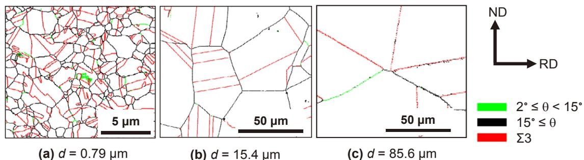
Fig. 1 Grain boundary maps of the cold rolled and subsequent annealed 31Mn-3Al-3Si TWIP steel: (a) 92 % cold-rolled and annealed at 700 °C for 0.3 ks, and (b) 92 % cold-rolled and annealed at 950 °C for 0.9 ks, and (c) 92 % cold-rolled and annealed at 1000 °C for 3.6 ks. The average grain sizes are also indicated.
