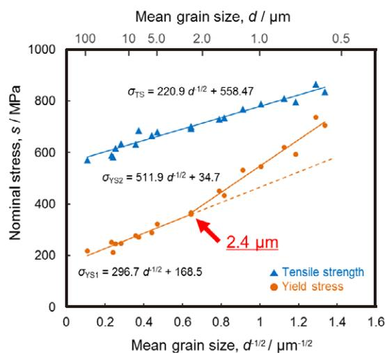
Fig. 3 Yield stress and tensile strength of the 31Mn-3Al-3Si TWIP steel plotted as a function of inverse square root of the mean grain size (Hall-Petch plot).
