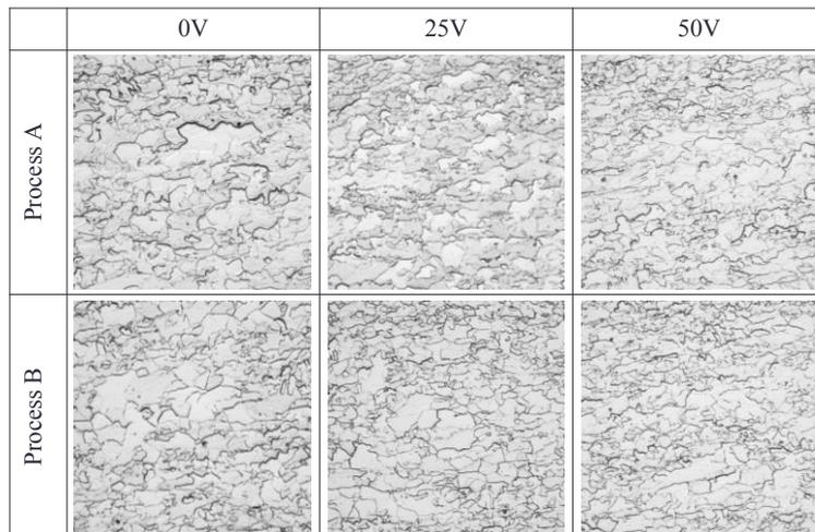
Fig.2 Optical Micrographs of the steels
