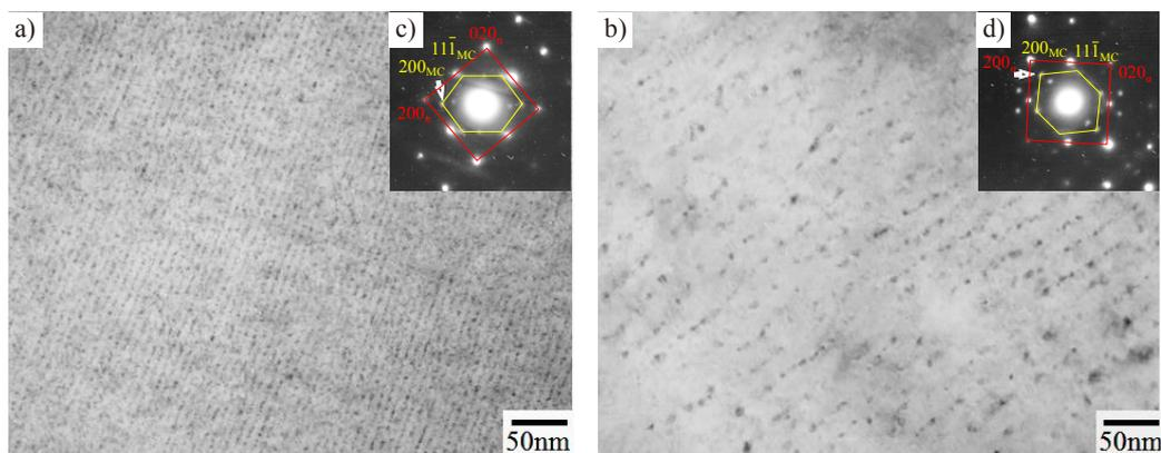
Fig.5 TEM micrographs of 25V steels (beam direction is parallel to  $[100]_a$ ) a) bright field image of process A, b) bright field image of process B, c) diffraction pattern of process A, d) diffraction pattern of process B
