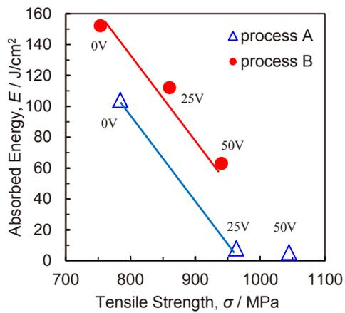
Fig.4 The balance of tensile strength and Charpy absorbed energy of the steels
