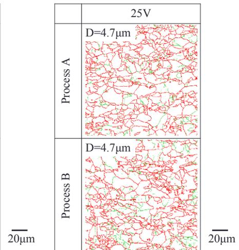
Fig.3 Grain boundary map of 25V steels by EBSD (misorientation angle: green line 5-15deg., red line >15deg.)
