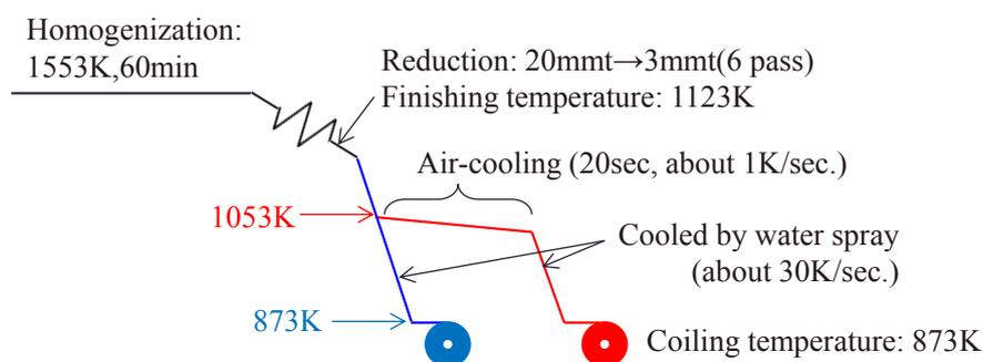
Fig.1 Schematic illustration of hot rolling and cooling conditions (A) 1-step cooling to 873K , (B) air-cooling from 1053K
