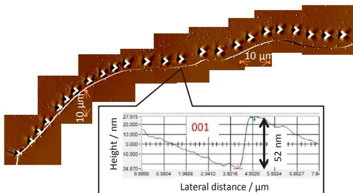
Fig.2 Scanning probe microscopy image of the sample surface after multiple indentations and the cross-section profile among the grain boundary.
