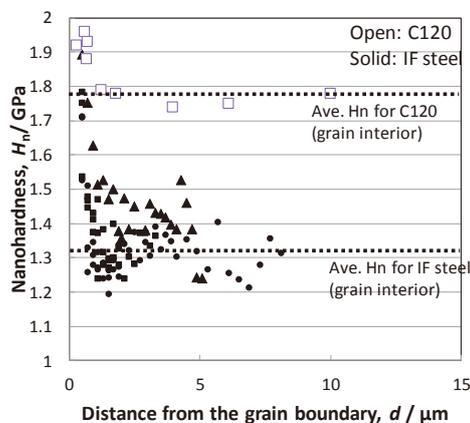
Fig.4 Relationship between nanohardness and the distance to the grain boundary.
