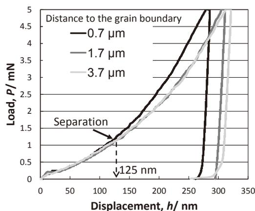
Fig.3 Load-displacement curves for the IF steel with different distances to the grain boundary (0.7, 1.7 and 3.7  $\mu\text{m}$ ).
